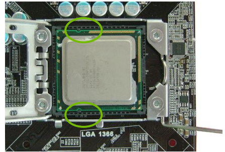
Align notches with notches on the CPU
