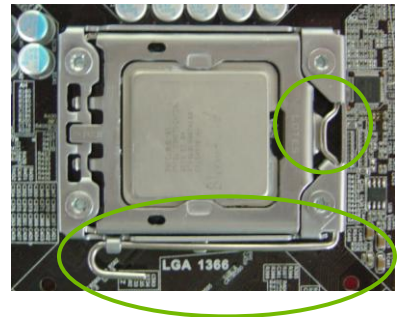
Align notches with notches on the CPU
