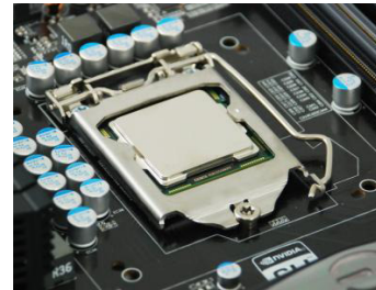
Align notches with notches on the CPU
