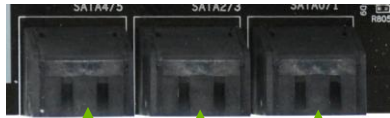
SATA 4 (bottom) SATA 2 (bottom) SATA 0 (bottom) SATA 5 (top) SATA 3 (top) SATA 1 (top)
