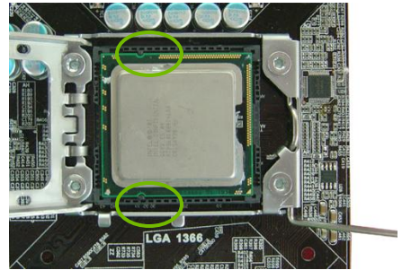
Align notches with notches on the CPU
