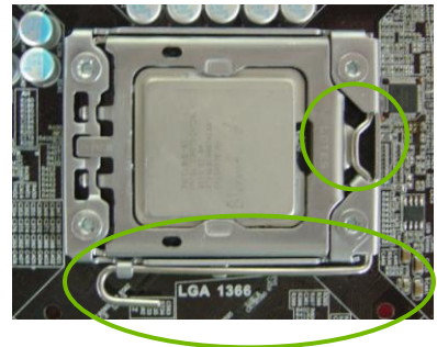
Align notches with notches on the CPU
