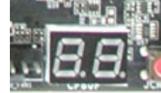
Debug LED with CPU Temperature Monitor
