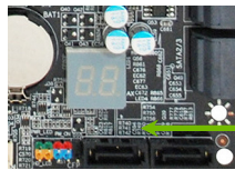
Debug LED with CPU Temperature Monitor
