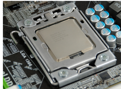
Align notches with notches on the CPU
