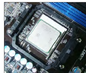
Align notches with notches on the CPU
