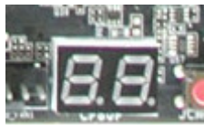
Debug LED with CPU Temperature Monitor
